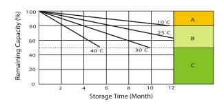
No supplementary charge required (carrry out supplementary charge before use if 100% capacity is required)
