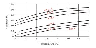
**Temperature Effects in Relation to Battery Capacity**
